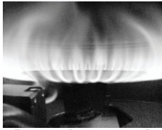
Proper burner and pilot burner pattern.
